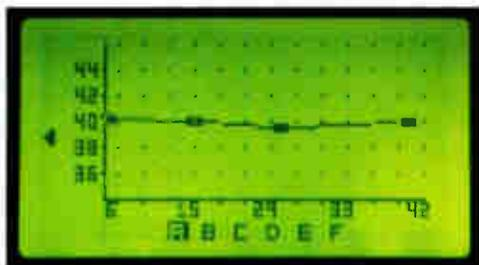
*When equipped with the Multiplexer Option, the 9580SST accepts signals from up to 8 separate test points and analyzes sweep & ingress from each individually, returning data to as many as 6 SSR field units (A thru F) connected to it.*
