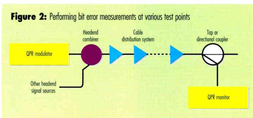
tions or faulty passive elements. Use a spectrum analyzer to look at the shape of the digital signal's spectrum and verify that it matches the shape seen at the headend. Look for new notches, ripples or asymmetry.
