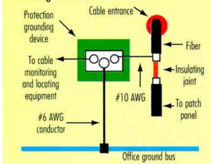
use of an "insulating joint" the outside plant cable can continue to be run into the office. This method eliminates the need for a splice enclosure at the building entrance. Local fire codes can be met by installing the cable in conduit. (See Figure 1.)
