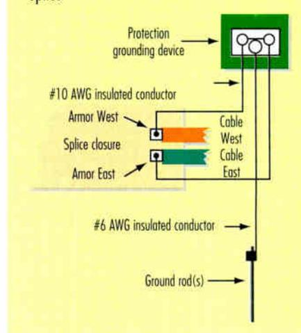
and sheath monitoring is to bond the armors to ground through a protective device in an accessible housing either above or below grade. A number of these enclosures are available on the market and allow for good cable maintenance practices. (See Figure 2.)
