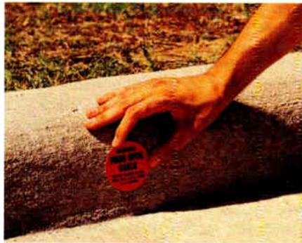
or sides of a curb, using a one-part adhesive. These resilient curb markers provide a warning to utility companies and contractors of the presence of underground fiber-optic or CATV lines. Cable routes and road crossings can be permanently marked with these low profile markers instead of a more obtrusive sign and post.
