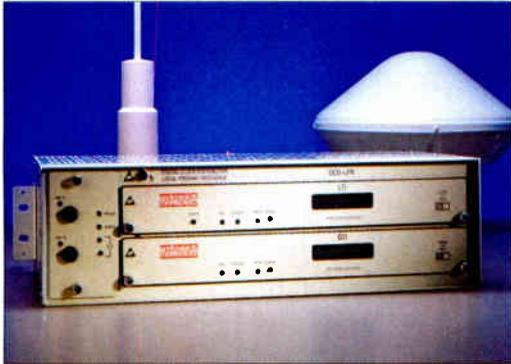
Local Primary Reference system using GPS and/or LORAN-C technologies.
