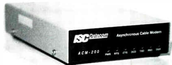
Model ACM-200 Asynchronous Cable Modem is designed to operate at any data rate up to 19.2 kbps, protocol transparent. This modem meets NEMA traffic control temperature requirements and is well suited to many data applications. FSK modulation provides reliable data transfer under severe noise conditions.
