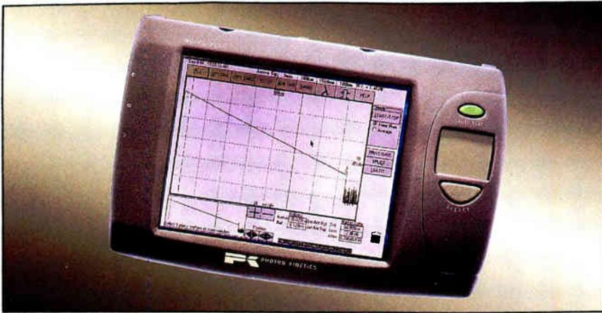
Take advantage of our continuing efforts to enhance the Model 7500 Mini-OTDR. 34dB of dynamic range and modular architecture make it both powerful and versatile.
