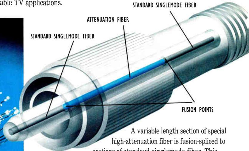
A variable length section of special high-attenuation fiber is fusion-spliced to sections of standard singlemode fiber. This reduces reflections, minimizes cladding effects, and eliminates epoxies from the optical path. It also allows connectors to mate to standard fiber:
