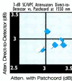
Consistent attenuation is achieved either with patch cables or when connected directly to the detector. The attenuator element does not strongly guide cladding modes that would produce different loss values when connected with or without a patch cable.
