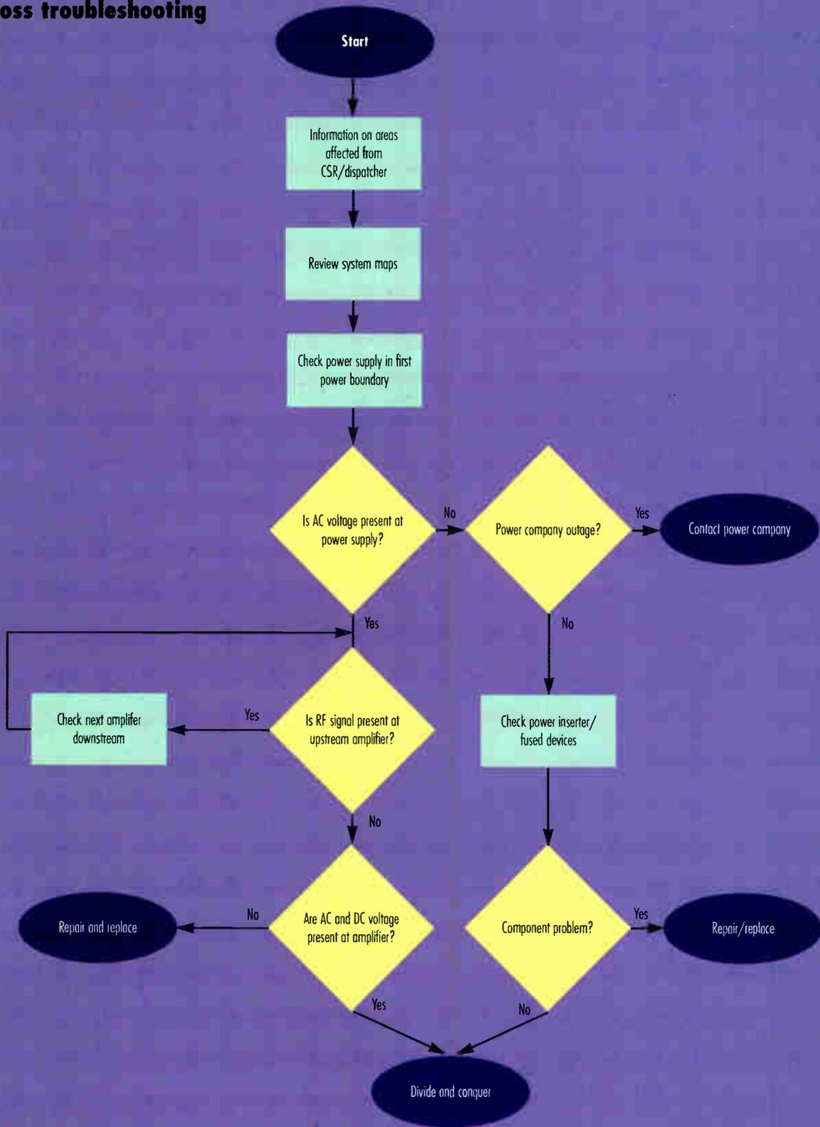
pinpoint a fault. A span of cable containing a short also can be identified by measuring amperage draw with a VOM. Apply the divide and conquer method to again save time and energy. Once the span has been identified, the TDR and/or leak detector
