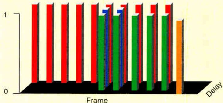
Upstream TDMA channel occupancy is typified by time domain sampling of subscriber traffic at all active electrical path lengths. This occurs within a single data frame. Thus, dynamic channel equalization is rendered more difficult. (Note: Sample density not to scale.)
