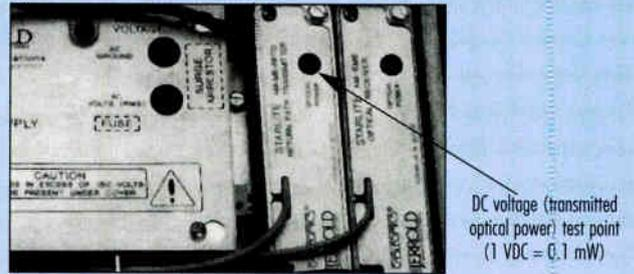
Figure 3A contains the formula for calculating the optical power level at the output of a return path transmitter with a 1 VDC/0.1 mW ratio using that transmitter's DC test point voltage. To calculate the optical output power in dBm using a DC test point voltage of 4 VDC, follow the calculations in Figure 3B: 1) multiply the measured DC voltage times 0.1 to obtain a quotient; 2) calculate the log of that quotient to obtain a resultant; and 3) multiply that resultant by 10.
