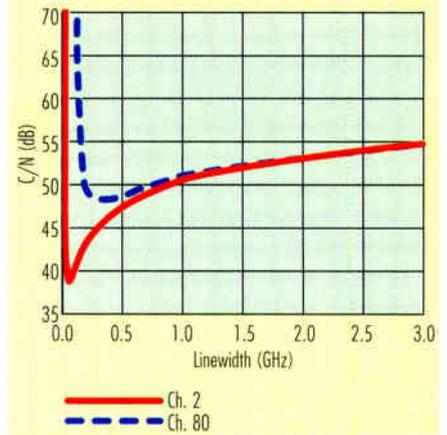
dB, and that reflections of about -30 dB are required to reduce C/N to levels near the cable TV limit of 50 dB. In most cases, if discrete reflections are kept below -40 dB—which is the specification for most commercially available splices and connectors—C/N degradation should not be a concern.
