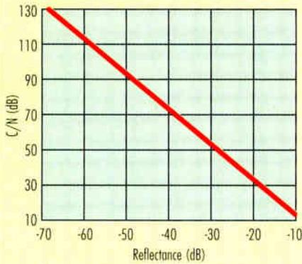
**Figure 2:** C/N from noise due to double Rayleigh backscatter
