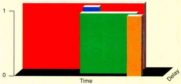
An OFDMA channel is typified by contiguous occupancy along the time axis, at a bulk delay that corresponds to the subscriber's electrical path length. Constant bulk delay "per channel" simplifies upstream dynamic equalization over the entire band.
