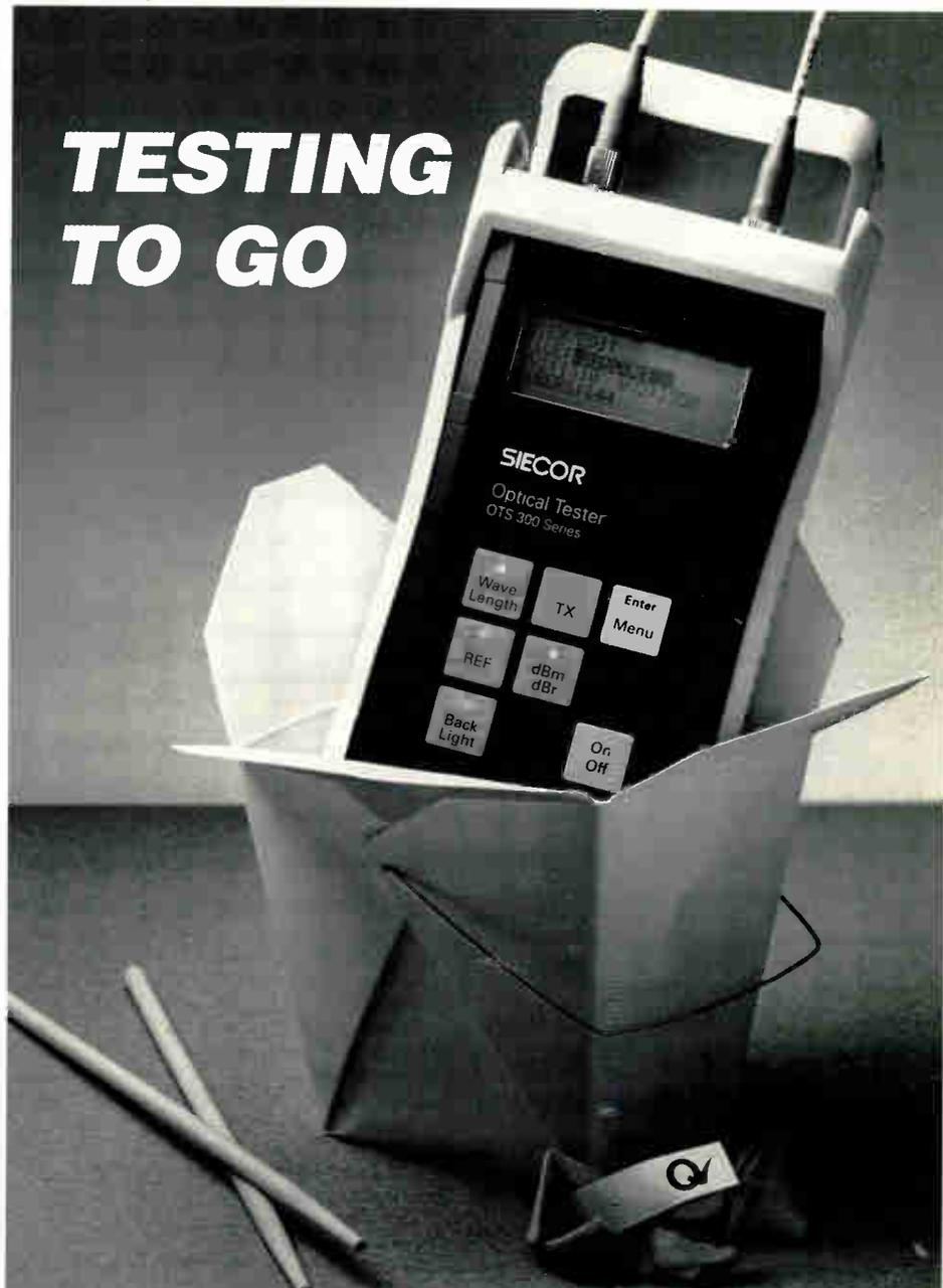
Siecor's OTS-300 Express Series Optical Test Sets get results quickly, especially with high count, bidirectional, dual wavelength testing. From the first reference to final printed results, simultaneous testing and data storage saves time and eliminates errors. The Express Series' intuitive operation, flexible Windows-based PC software,
