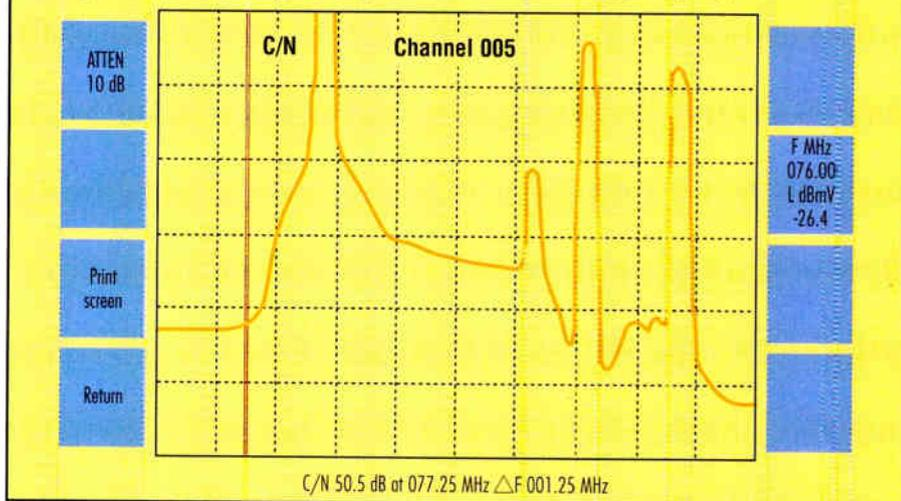
**Figure 2:** Screen capture of C/N measurement method (Example 2)
