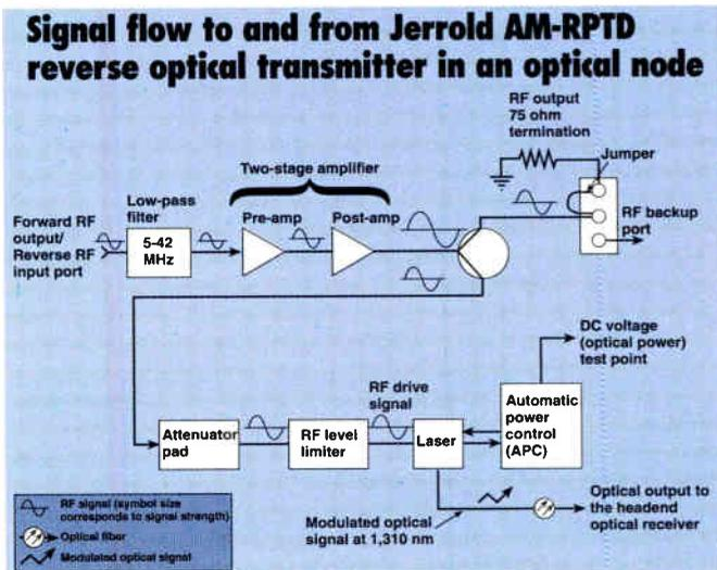
(approximately 6 dB) by a two-stage amplifier. The amplified signals are then split, with one signal routed to the RF backup port for operational redundancy. This signal is normally terminated inside the node. The other signal is routed through an attenuator pad to reduce the signal level. The reverse RF signals are then routed to an RF level limiter, which protects the laser against an RF input signal level exceeding +15 dBmV.
