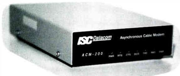
Model ACM-200 Asynchronous Cable Modem is designed to operate at any data rate up to 19.2 kbps, protocol transparent. This modem meets NEMA traffic control temperature requirements and is well suited to many data applications. FSK modulation provides reliable data transfer under severe noise conditions.
