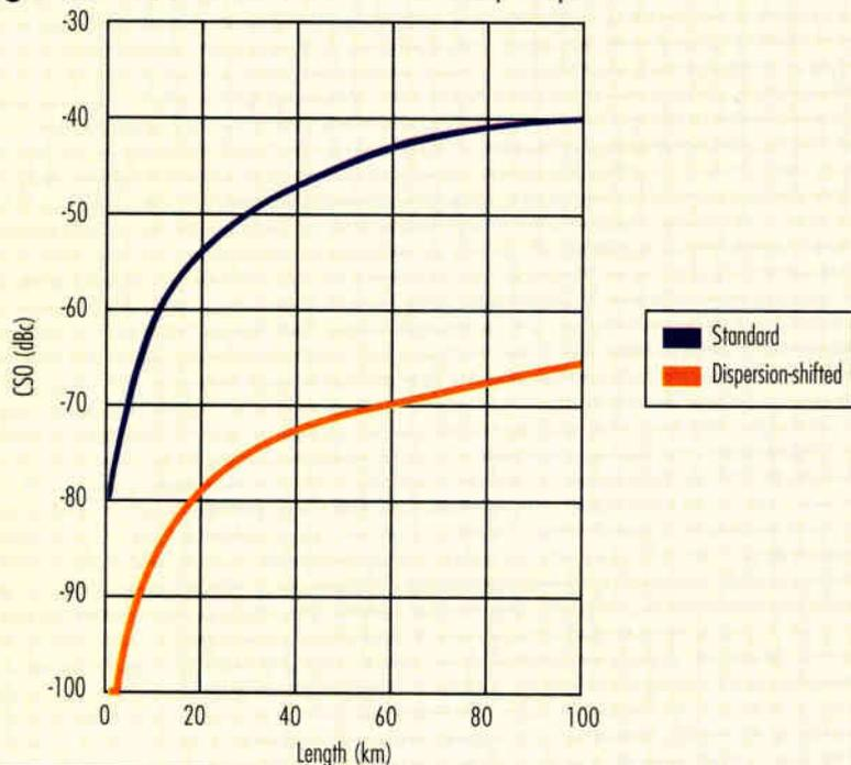
**Figure 3:** Theoretical calculations for self-phase modulation component
