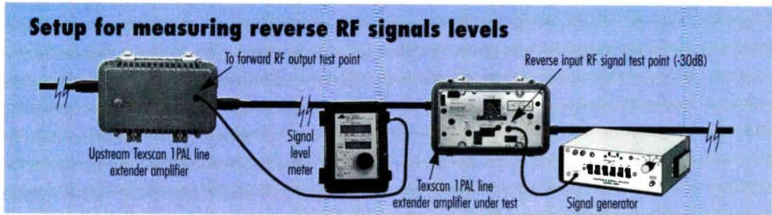
**D**etermining the proper reverse equalizer (EQ) value for a Texscan 1PAL 750 MHz line extender (LE) amp requires connecting test equipment, measuring reverse RF signals, performing calculations and selecting/installing the required EQ.
