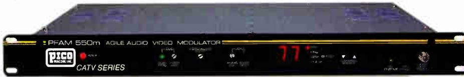
The **PFAM 550m** is a microprocessor controlled rebroadcast quality, phase locked loop synthesized, frequency agile CATV television modulator. The
