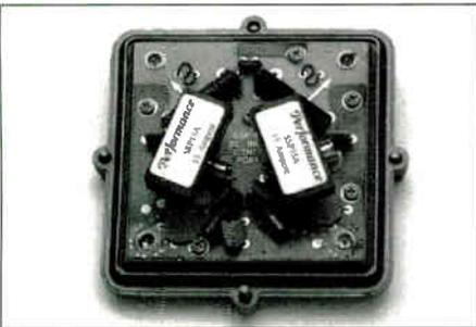
**SURGE-GARD protects against nuisance fuse blowing and resets in 60 seconds**
