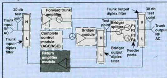
**Figure 3:** Block diagram of a C-COR return amplifier module
