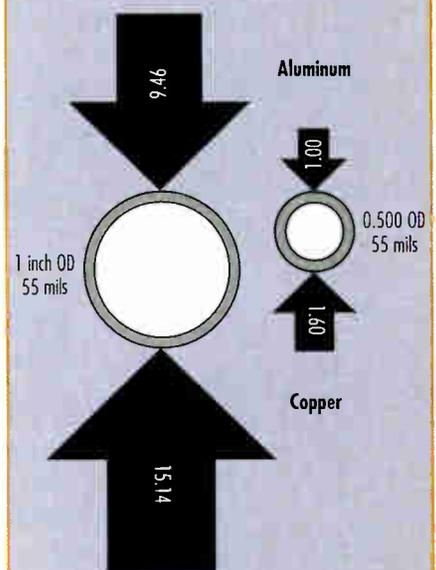
**Figure 3:** Comparative force to deflect aluminum tubes and wire
