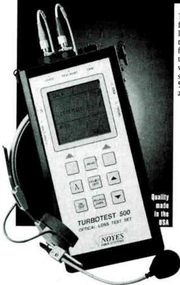
The new TURBOTEST 500 provides lightning fast, single fiber, bi-directional optical link loss, and optical return loss testing. Store up to 1024 dual wavelength measurements for future downloading to a PC or printer. Get the talk-set option, and you can communicate with your partner over an unused fiber to speed the testing process. The TURBOTEST 500 even functions as an optical power meter and stabilized laser source.
