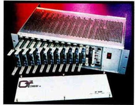
Olson Technology has introduced a compact, modular, frequency agile 12-channel remote control video headend system. The Olson OT-1200 series system features a 5.25- x 19-inch rack-mount housing that contains a power supply and can be configured with any combination of video/audio modulator or demodulator cards. The system operates at frequencies from 54 to 550 MHz and permits local tuning or remote control of each card via a serial data link.
