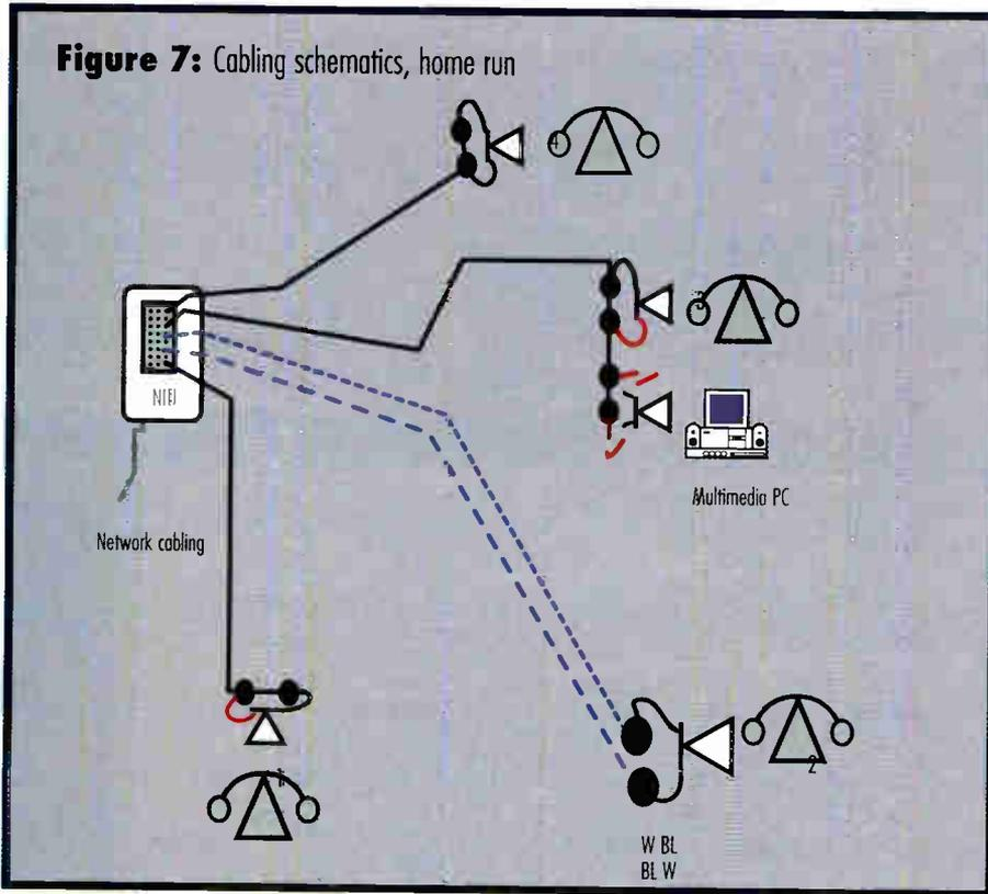
moves are easily completed because of the physical appearance of the wiring at a single outlet in the home run or star wired distribution associated with today's 110 system deployment. Rapid testing of services at each outlet is achieved since the outlet is easily identified at the service box location with inexpensive test equipment.
