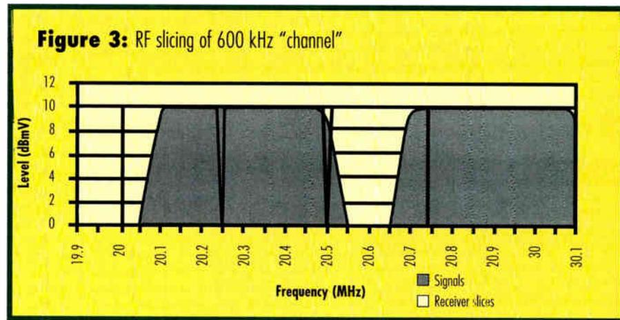
that it does not see anything from any adjacent channels. Frequently, however, this is not possible. To measure our test signal, a RBW between 4 and 6 MHz would get us fairly close to the right answer, but most spectrum analyzers limit RBW to 3 MHz maximum.
