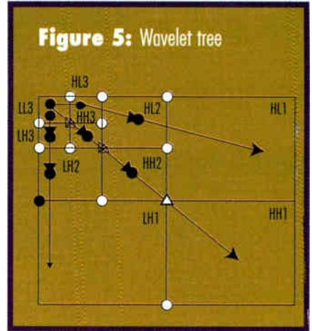
wavelet coefficients are represented by a structure known as a wavelet tree, in which the nodes of the tree correspond one-to-one with the wavelet coefficients. The coefficient at the coarse scale is called a parent, and all coefficients at the same spatial location and of similar orientation at the next finer scale are that parent's children. Figure 5 shows such a wavelet tree with three levels of decomposition.
