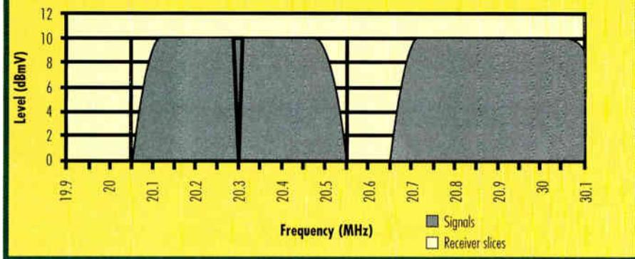
measured are at 600 kHz spacing with 50 kHz internal guardbands on each side, and the RF "slices" are 250 kHz each. If the meter is programmed with a 600 kHz channel centered at 20.3 MHz, it needs to take three slices to cover the band completely, and measures a total bandwidth of 750 kHz. If there is a guardband next to the signal to be measured, this is OK, but extra power may be measured if another signal is in the
