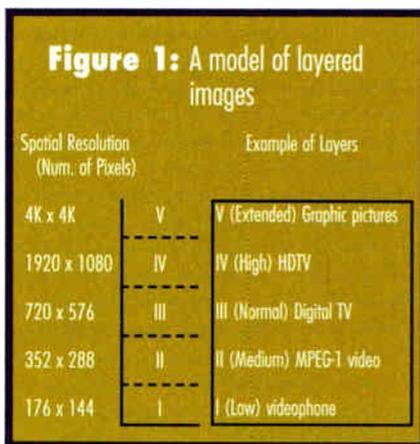
This layered coding gives users more freedom to select the quality level they need. The conceptual table in Figure 1 categorizes layers into spatial resolutions ranging from video telephone image (which can be as small as 176 x 144 pixels) to high-resolution graphics or medical images (which can be as large as 2,048 x 2,048 pixels).
