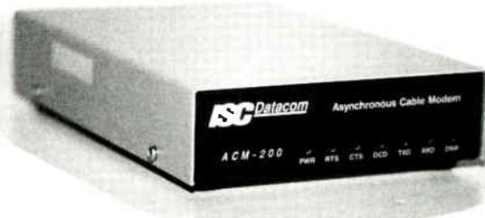
Model ACM-200 Asynchronous Cable Modem is designed to operate at any data rate up to 19.2 kbps, protocol transparent. This modem meets NEMA traffic control temperature requirements and is well suited to many data applications. FSK modulation provides reliable data transfer under severe noise conditions.
