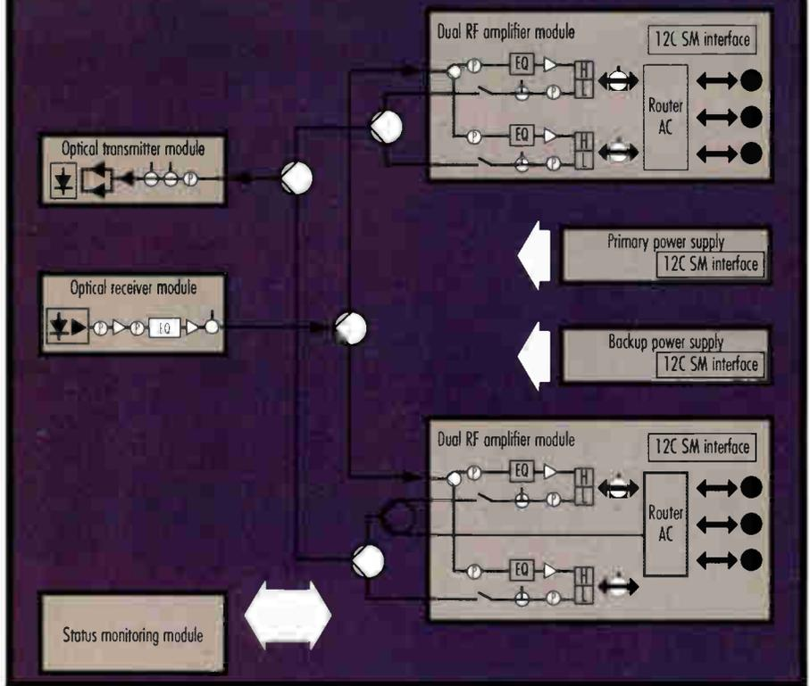
**Figure 2:** A node with analog video and 4 Mbit/sec. data service.
