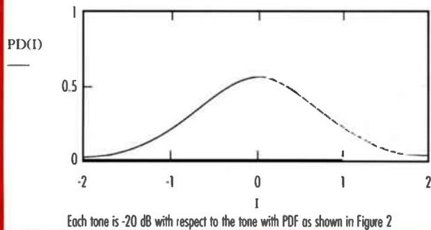
Now let's assume that one of these carriers is to be replaced with 100 lower level narrowband telephony carriers. If the constant power design rule is applied, the level of each of these carriers should be 20 dB below the level of each of the five tones used to characterize the laser. This would result in the same average composite power applied to the laser.
