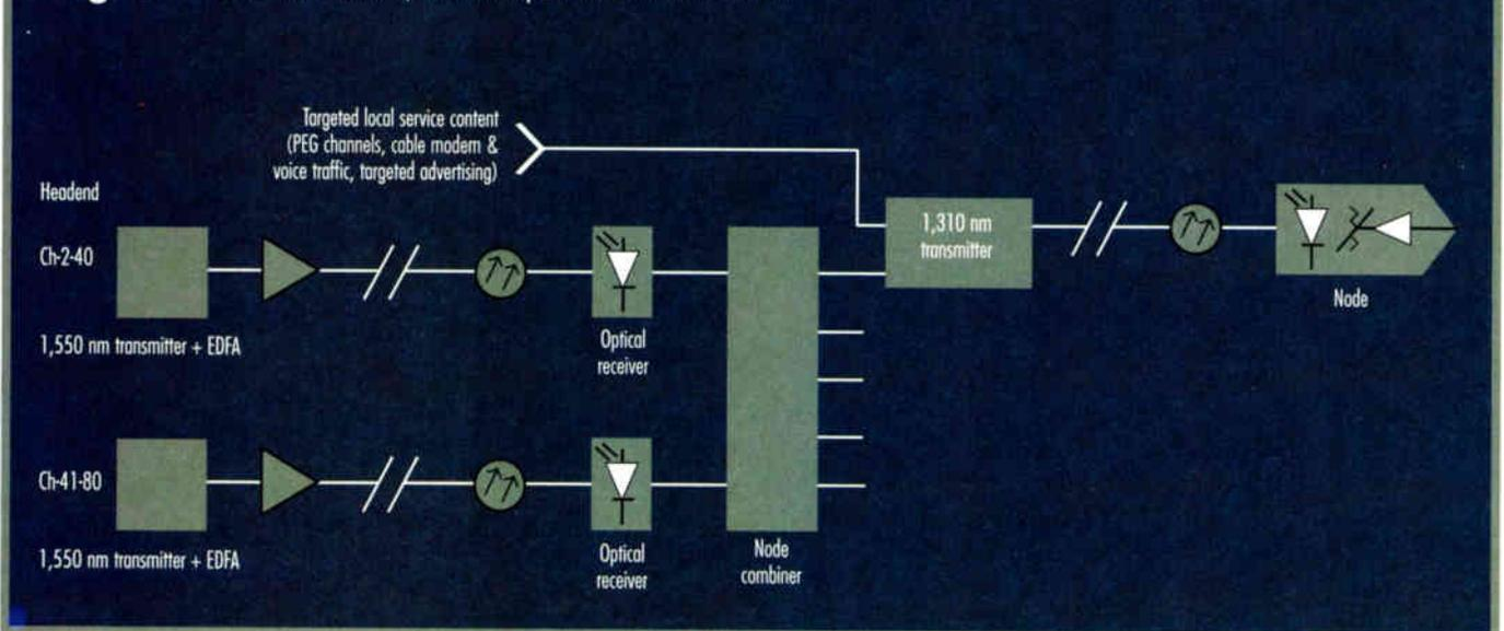
dBm output power) boosts the signal. A high-count optical splitter network then divides the signal to provide the appropriate node count, link loss budget and received power at the node.
