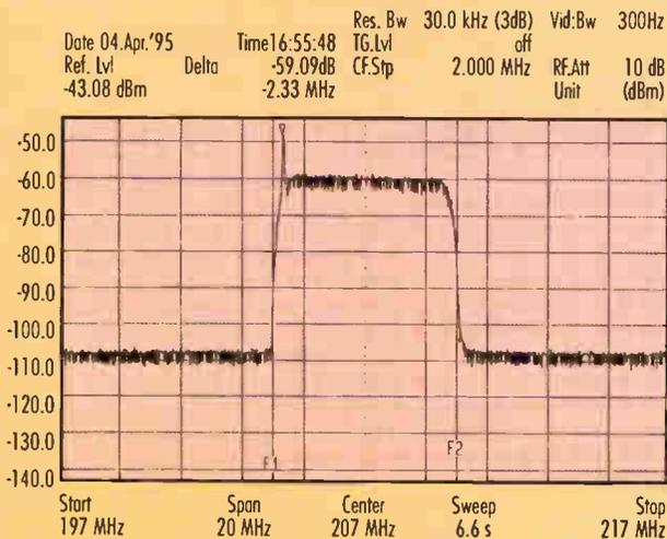
**Figure 2: 64-QAM signal in the frequency domain**
