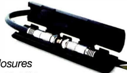
Designed for direct burial, gel-filled CERTI-SEAL closures protect F-connector splices. Their one-piece design snaps together for easy assembly, and to eliminate lost parts. Innovative centering tabs and a molded-in strain relief reduce the possibility of temperature-induced movement.
