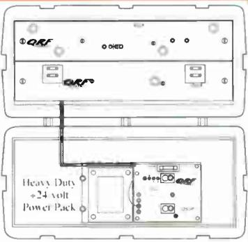
This system of modules, chassis and positive voltage power pack replaces the contents of SJ housings for drop-in upgrade to 550/600!
