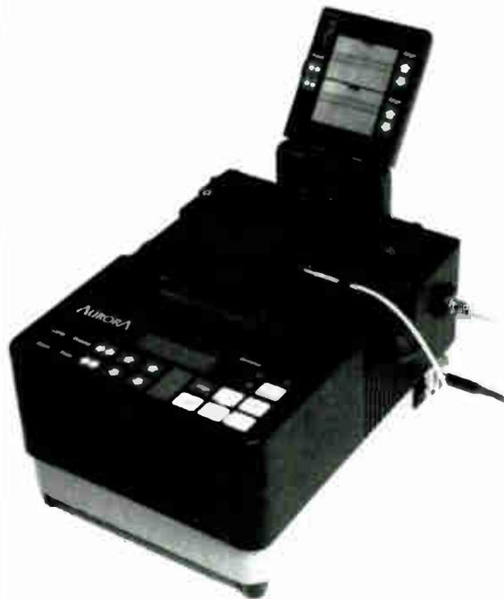
**A**t Aurora Instruments, Inc. we think you should. We've taken the guesswork out of splicing by using the most advanced active alignment system available in our family of fusion splicers. Active optical alignment enables you to obtain the lowest splice loss and most accurate loss estimate possible.
