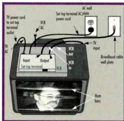
Figure 2: Hum bars present when set-top terminal reconnected indicate a defective set-top
