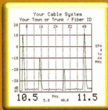
RDU's monitors ingress and noise, where you designate, by selecting up to 200 frequencies from 4 to 44 MHz. The RDU averages the energy and displays CRI's exclusive I-NAN number.
