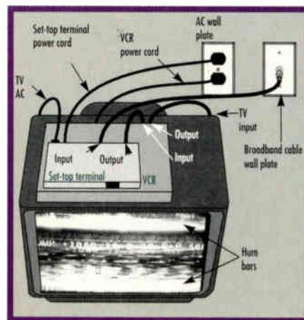
Figure 3: Hum bars present when VCR reconnected using known good set-top terminal indicate a defective VCR
