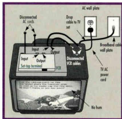
Figure 1: No hum on TV set when connected directly to the wall plate
