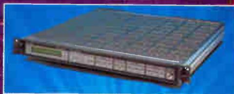
PULSAR modulators provide complete software control, allowing you to monitor and manipulate all modulator functions from a central location. In the event that lost or degraded signal is detected, you can remotely route the signal to a back-up modulator without the expense or delay of dispatching a technician to the headend.
