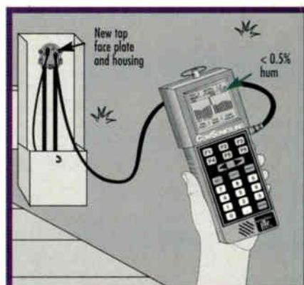
Figure 4: Measuring acceptable hum after replacing tap face plate and housing
