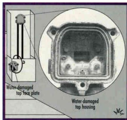
Figure 3: Water-damaged tap causing unacceptable hum
