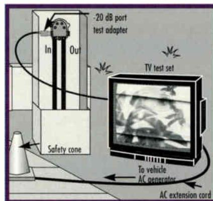
Figure 2: Checking picture quality at tap input using test port adapter and TV test set
