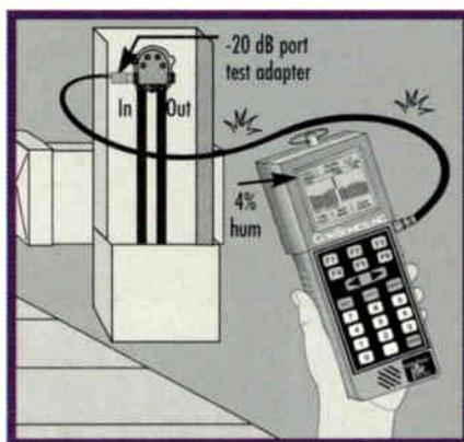
Figure 1: Measuring hum at tap input using test port adapter and SLM
