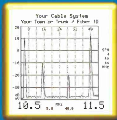
The RDU measures Ingress and Noise, where you designate, by selecting up to 200 frequencies from 4 to 44 MHz. The RDU averages the energy and displays CRT's exclusive **I-NAN<sup>®</sup>** number.
