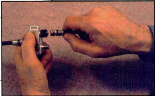
Step 9: For all outdoor connectors, install a thread-sealing sleeve on the mating connector port. Then hand-tighten the connector on the port.
