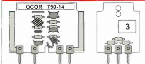
**NEW 750 MHz SEQ-style equalizers.** 0 dB to 24 dB in 2 dB steps. **QCOR750-14** for \$8.75. Our version of 750 MHz. **SPB-P** style of C-Cor pad values are from zero to 20 dB in 1 dB steps. Order our **QCOR-P** and replace the asterisks with the dB value. only \$5.00 each.
