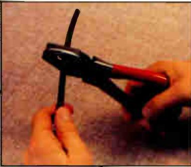
*Step 1: Squarely cut the end of the cable with a sharp pair of wire cutters.*
