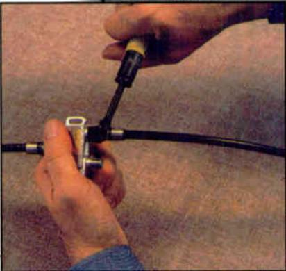
Step 10: Torque the connector nut to between 20 and 30 inch-pounds. The torque wrench shown is factory preset to 30 inch-pounds. A word of caution: Do not use torque wrenches on consumer equipment such as TV sets or videocassette recorders (VCRs). The connectors on those devices may be damaged by tightening much beyond finger-tight.
