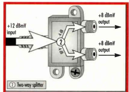
Figure 2: Insertion loss effects of two-way splitters
