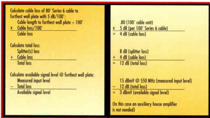
Figure 1: Calculating signal level at furthest outlet/wall plate
