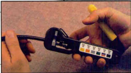
Step 7: Insert the cable and connector into the crimp tool. This particular tool is a compression-type crimper.
