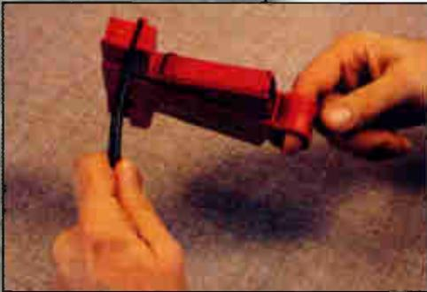
*Step 3: Rotate the tool around the cable three to five times. This will remove the correct amount of jacket and dielectric material.*
