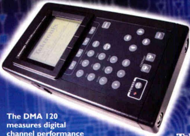
The DMA 120 measures digital channel performance in just a few keystrokes and provides information to efficiently install and maintain the cable network. Troubleshooting with the analyzer is aided by constellation, spectrum and equalization display modes.
