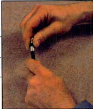
Step 6: Install the F-connector on the prepared end of the cable.
