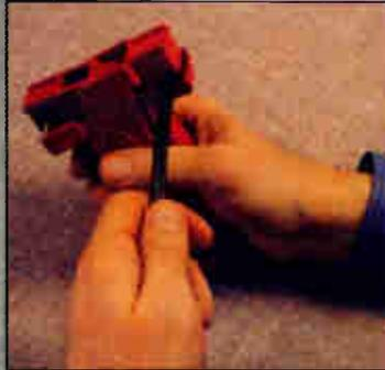
*Step 2: Next, insert the end of the cable in the cable preparation tool. This particular model features color-coded replaceable blade cartridges for 59, 6 and 11 series cable in the same tool.*
