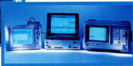
*HP Mini-OTDR HP Rack OTDR HP OTDR*
