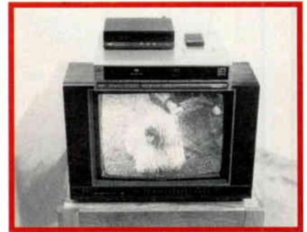
Figure 3: Picture effects of too low input signal to amplifier
