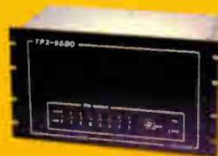
**The 9580-SST<sup>SM</sup>.** The SST headend unit collects balancing and ingress measurement data from one to eight test points, and transmits updated measurements to the SSR field units, the second component of the 9580 system. The SST operates as an ingress monitor, receiving 80 ingress samples per test point, per second.
