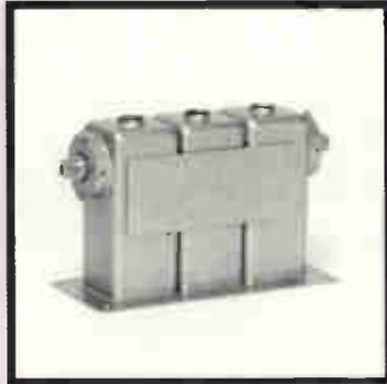
The filter achieves more than 15 dB rejection at  $\pm 8$  MHz from center frequency and more than 40 dB rejection at  $\pm 22$  MHz from center frequency. A minimum of 14 dB return loss is maintained in the passband. The filter can be tuned to any 6 MHz channel in the 470 MHz to 890 MHz range and comes in 50-ohm or 75-ohm configurations.
