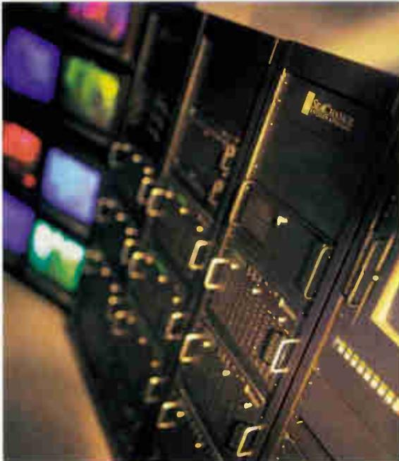
AT&T Cable Services has installed a five-node MediaCluster video server system to support its InnTelevision service. The system can store roughly 400 feature-length movies.
