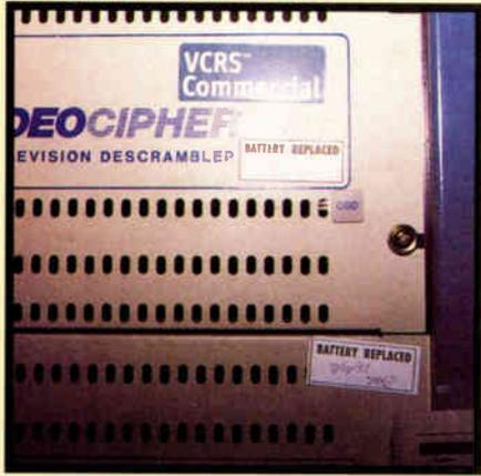
Keep track of battery replacement by labeling equipment with the date the battery was installed.
