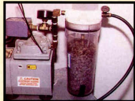
Make sure your dehydrator crystals are blue—indicating that the line gas is dry. Even a canister with half blue and half pink crystals is better than no moisture absorption at all.
