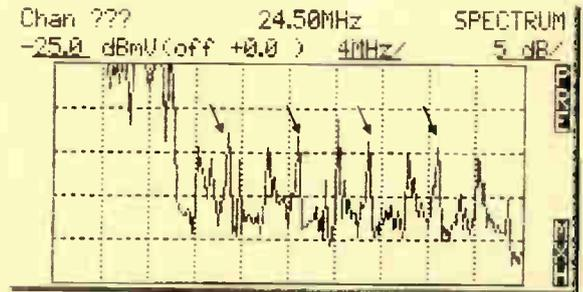
Figure 3, at bottom right, indicates common path distortion (CPD). The beats are spaced every 6 MHz (8 MHz for a phase alteration line, or PAL, system).
