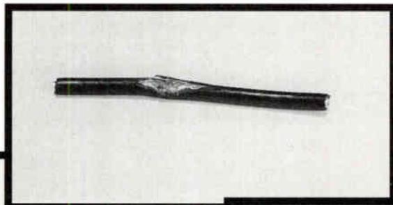
Still more possible sources of ingress and its results: Clockwise from bottom left, corroded connectors, a cracked crimp ring, severely scraped cable, and a distorted image. Photos courtesy of the NCTI
