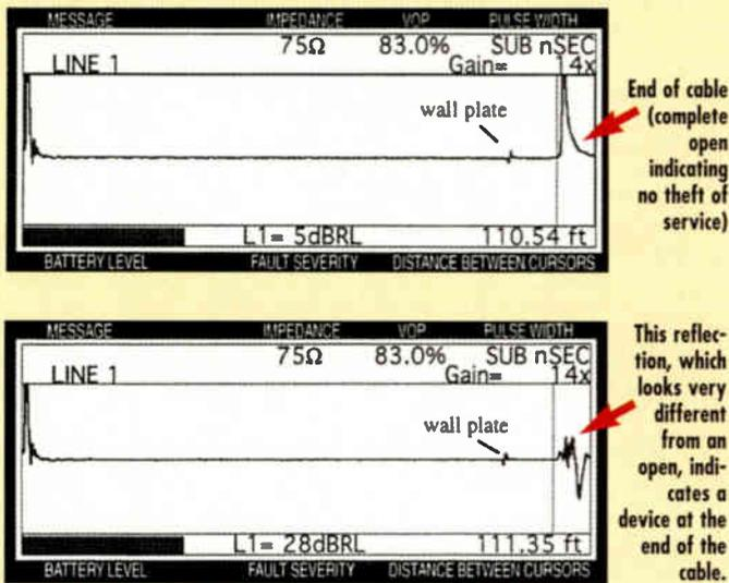
The top waveform shows a substantial upward reflection, which indicates a complete open (nothing reflected on the cable). This would indicate that the cable is not connected to a device such as a TV set or VCR. The bottom waveform is dissimilar from the first in that it indicates that a device is connected to the cable and that service theft could be occurring.
