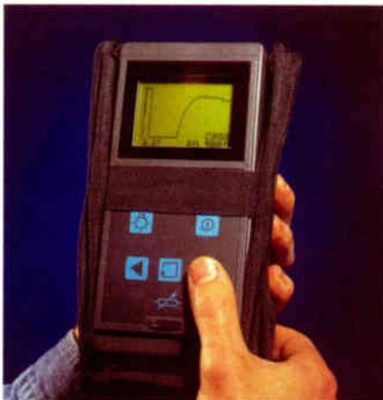
TDRs and OTDRs feature a variety of options for storing, analyzing, and displaying waveforms.
