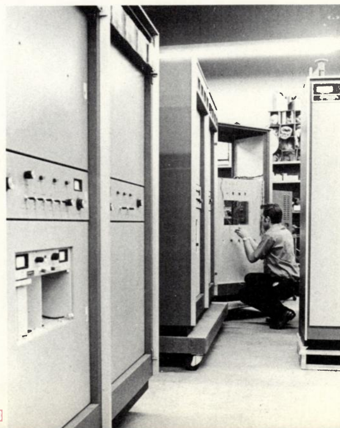
DICK NOTEMAN, Sparta Transmitter Production Leadman, works on a Model 660 FM Exciter Installation in a 603A5 Transmitter. The 660 is seen in the foreground, mounted in the model 620 20kw FM transmitter.
