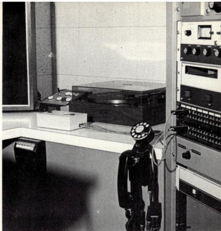
This partial view of the KZST production room shows (lowest in the rack) the SPARTA 25 Hz Oscillator-Filter (allowing reel transports to be programmed by the 1052 Controller), and just above the jack panel the 600-CRP Record/Playback with its Record Amplifier for producing commercials on cartridge. Next to the turntable, left of center, are SPARTA Remote Control sets for the reel-to-reel machine (not visible) and the 600-CRP. The production room operator has positive control of all recording equipment at his fingertips. The control board is at left, out of the picture, with the operator facing away from the camera towards the left. A second turntable is available on the matching left-hand wing of the console desk.
