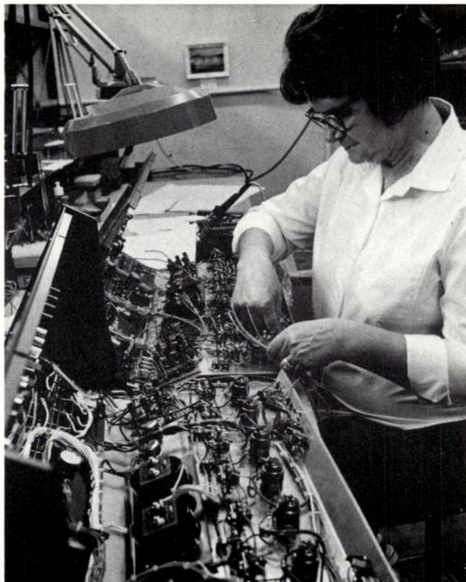
Assembler EDITH GRAHAM wires the fore-panel of an AS40B 8-channel stereo console on the Sparta production lines. Most of the exacting handwork is done by women.
