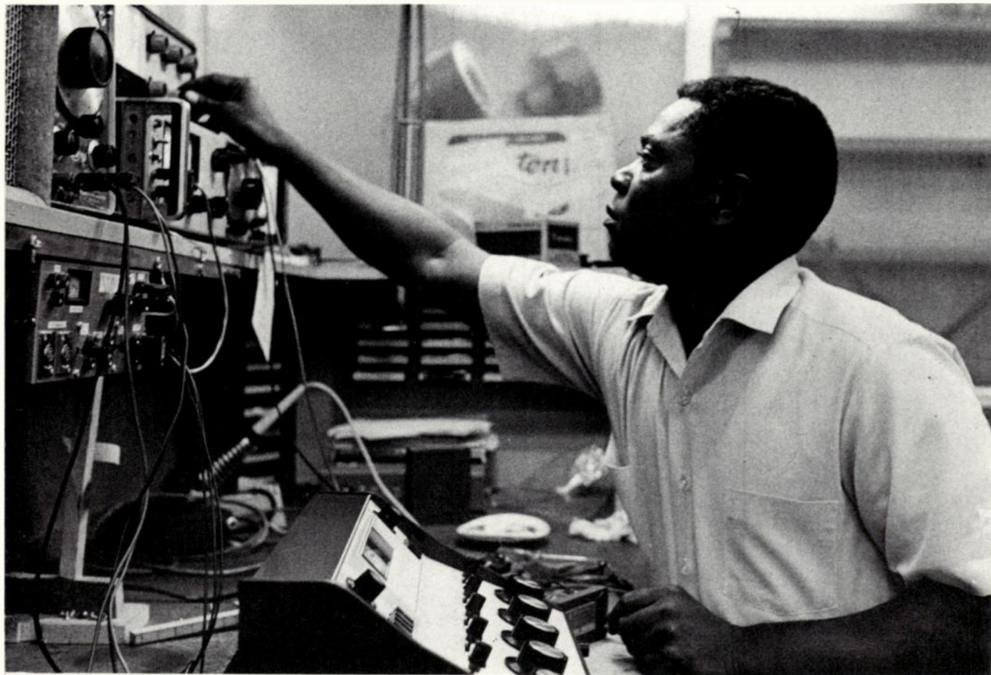
In final checkout each electronic component and assembled unit is tested for its exact characteristics, which information is furnished to the buyer. RICHARD McGEE, Technician, checks output of an A15B 5-channel monaural console.
