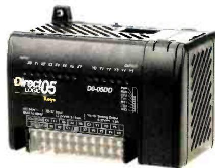
A Direct Logic PLC, featuring eight logic inputs and six relay outputs
