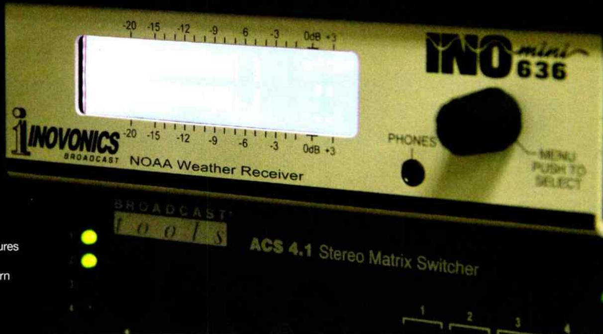
The front panel features a monochromatic screen, one push/turn selector knob and a headphone jack.
