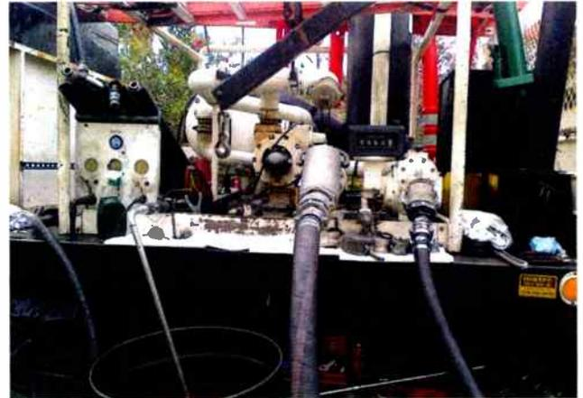
Fig. 3: This photo shows a truck-mounted fuel polishing system.
