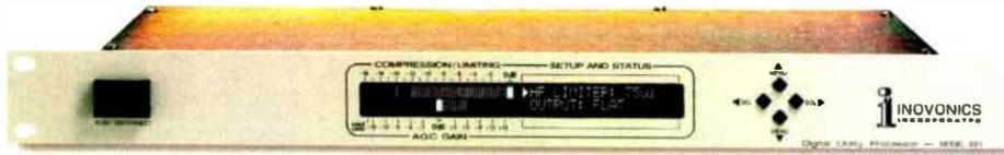
In addition to AGC the 261 has emphasis limiting, making it a good choice for protecting radio STLs.
