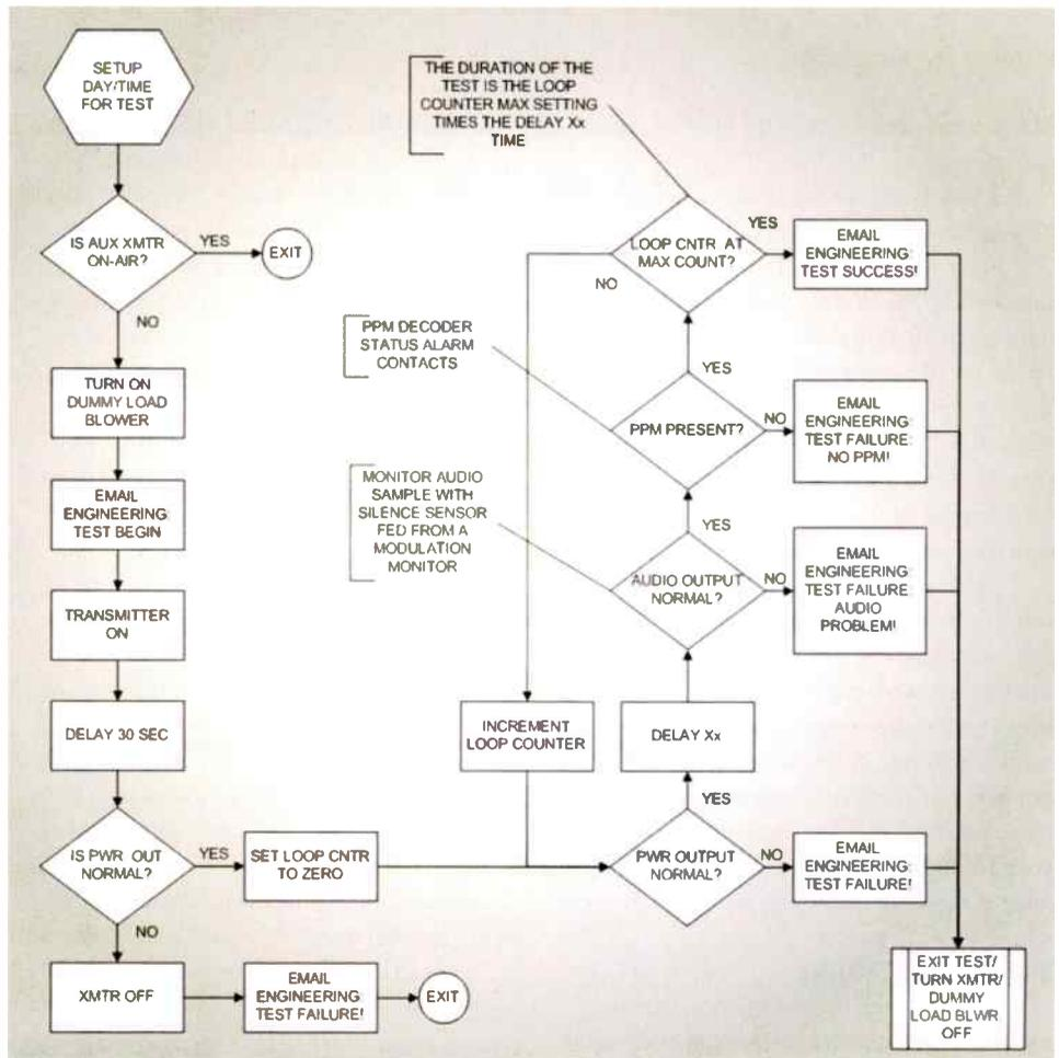
This is an example of a transmitter test routine.
