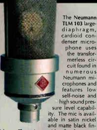
ishes. The mic provides flat frequency response to 5kHz with a 4dB presence boost in higher frequencies. It is capable of handling sound pressure levels up to 138dB. The K 103 large diaphragm capsule is based on the K 87, well known from the U 67/U 87 microphones.
