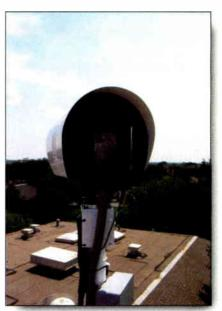
FSO links are proving to be practical and do not require frequency coordination. Photo courtesy of Lightpointe.
