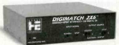
**DigiMatch 2X6** converts digital audio between AES/EBU and SPDIF. It's also a **digital DA**, with six digital audio outputs!
