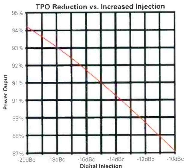
Figure 3. Output power reduces as digital injection increases.
