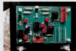
This is a direct replacement for the PR&E CI-2 interface. Use where OPTO ISOLATION is needed between your device and console logic. Each module comes with connectors, pins and instructions. Optional mounting panel for 8 modules and 2 Warning Light relays.
