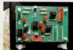
This is a direct replacement for the PR&E CI-2 interface. Use where OPTO ISOLATION is needed between your device and console logic. Each module comes with connectors, pins and instructions. Optional mounting panel for 8 modules and 2 Warning Light relays.
