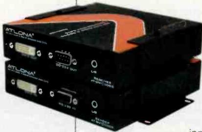
The receiver modules then convert that twisted pair signal back into the DVI with stereo audio and RS-232 data signal. The AT-DVI100SR is capable of extending signal up to 330' while the AT-DVI250SR extends signal up to 825'. In these lengths, each of the DVI extenders is still capable of maintaining high video resolutions up to 1920x1200 or 1080p, and they are entirely HDTV compatible.
