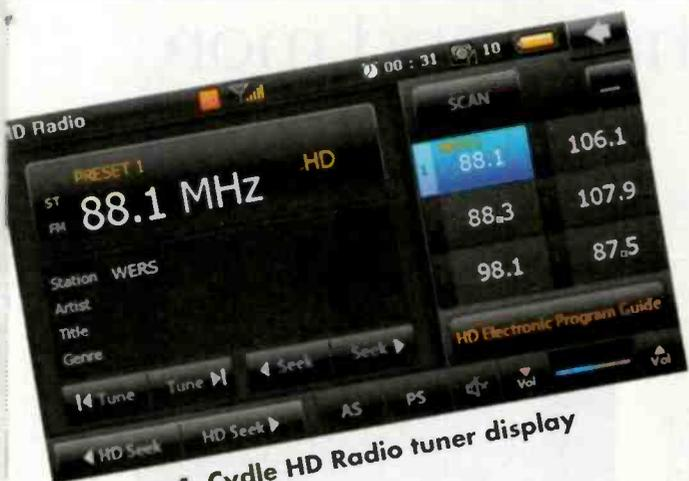
Figure 4. Cydle HD Radio tuner display with EPG feature
