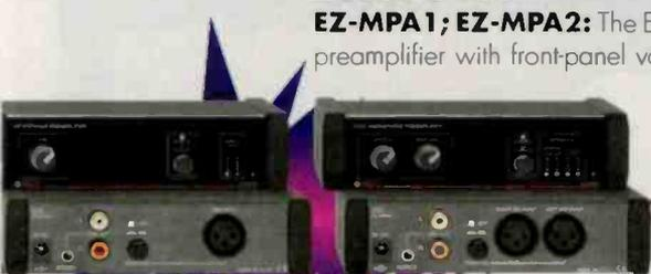
**EZ-MPA1; EZ-MPA2:** The EZ-MPA1 is a microphone preamplifier with front-panel volume control and audio level metering. A front-panel switch engages an audio compressor to control overloads and clipping during high-level audio bursts or peaks. Dynamic or condenser microphones are both supported with rear-panel switchable phantom voltage. The preamplified mic signal feeds both channels of the line output on RCA or mini jacks. LED VU metering facilitates easy level adjustment.
