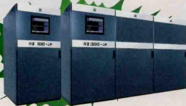
**NX Series:** With power outputs ranging from 25kW to 2000kW, this transmitter series offers AM adaptive pre-correction, ac to RF efficiency of 90 percent, linearity utilizing a nine-phase Direct Digital Modulation scheme encoded at 2.7 mega-samples per second, and a footprint requiring 1/3 to 1/2 less space than other transmitters. A touch-screen controller plus remote Web access are standard.
