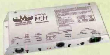
**MLM:** The Musicam USA MLM is a high quality limiter for microphone or mono line limiting applications. The limiter has a complex programmed dependent attack and release time system which is coupled with FET gain reduction to give a clean sound, free of the harshness often associated with VCA based designs.
