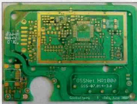
**Board of FM receiver with internal antenna**
