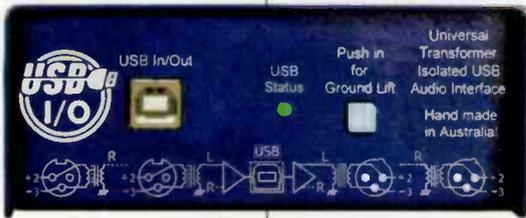
**USB I/O:** The ARX USB I/O is a plug-and-play USB digital/analog pro audio interface that removes the need to use any existing sound card outputs. It features full transformer
