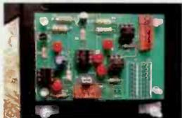
This is a direct replacement for the PR&E CI-2 interface. Use where OPTO ISOLATION is needed between your device and console logic. Each module comes with connectors, pins and instructions. Optional mounting panel for 8 modules and 2 Warning Light relays.
