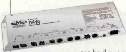
**DA14:** The Musicam USA DA14 is a versatile distribution amplifier capable of simultaneous distribution of both stereo and mono audio at a wide range of levels. Both balanced and unbalanced loads
