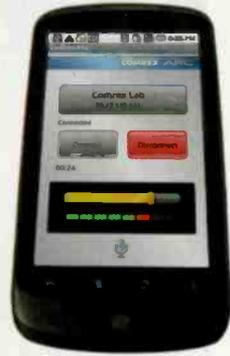
ARC is free. Access and Bric-Link customers with a Comrex-approved Android phone can download the application and connect via the phone's 3G or Wi-Fi to their Access or Bric-Link codec.
