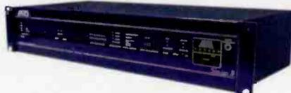
**DDA-416/WC106:** The Model DDA-416/WC106 is an integrated package containing four 1x4 AES/EBU digital audio distribution amplifiers and one 1x6 clock distribution amplifier. Operation of the unit is simple and straightforward, and it is housed in a rugged 2RU enclosure. All audio connections are made directly to the unit's built-in XLR and BNC connectors, and no special breakout cables are required. Signal routing is provided via rear-panel DIP switches.
