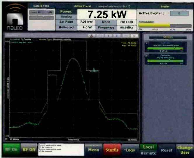
**Figure 2. The spectrum display of a Nautel NV10 running asymmetrical sidebands.**
