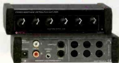
**EZ-HDA6:** The EZ-HDA6 contains six stereo headphone amplifiers with individual front-panel volume controls. Headphone outputs are provided on rear-panel 1/4" jacks. One input signal feeds all the amplifiers. Stereo RCA jacks, a mini jack and a dual 1/4" jack (for loop out connection) are provided for connecting the input source.
