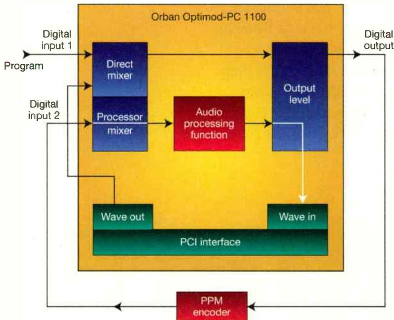
**Figure 1. Handle all streaming ad insertion using a sound card such as the Orban Optimod-PC 1100 (or 1101).**
