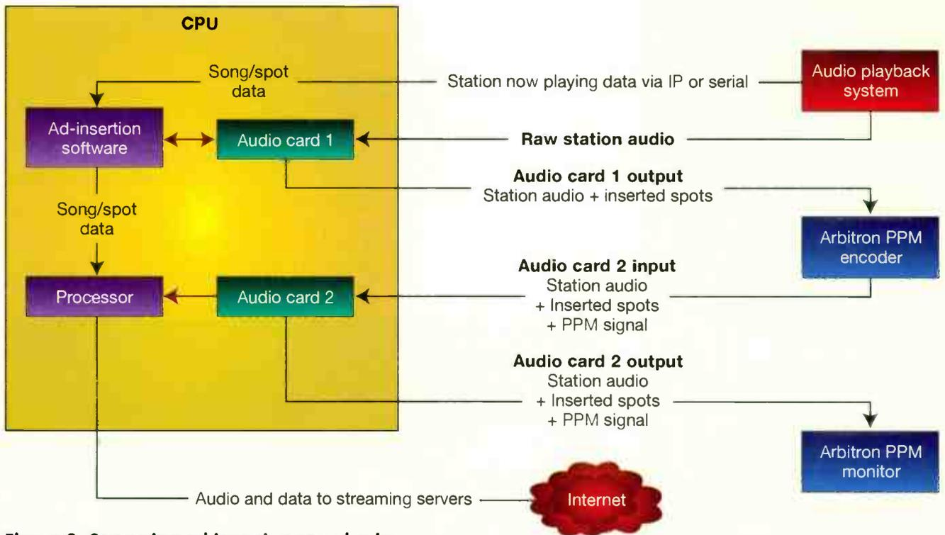
**Figure 3. Streaming ad insertion can also be accomplished using Liquid Compass Radius Live with Ando Media, as seen here.**
