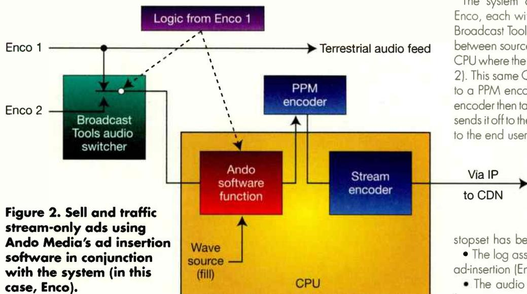
**Figure 2. Sell and traffic stream-only ads using Ando Media's ad insertion software in conjunction with the system (in this case, Enco).**
