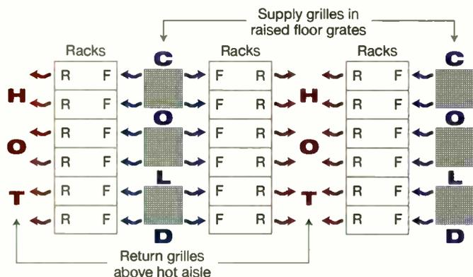
**Figure 1. Ideal placement of cold air supply and hot returns in a rack room.**
