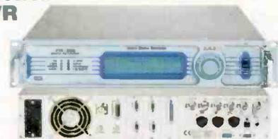
**PTX100-DDS:** PTX100-DDS uses DSP technology complying with all EC, FCC and CCIR standards. It features a built-in digital stereo coder, ITU professional limiter and on-board RDS, and AES/EBU, L/R, mono and MPX inputs, auxiliary inputs for SCA/RDS signals. It is completely microprocessor controlled, easy to program via menu or RS-232, and all main parameters are displayed on the LCD screen. It interfaces with all RVR telemetry systems to guarantee simple remote control of operating parameters.
