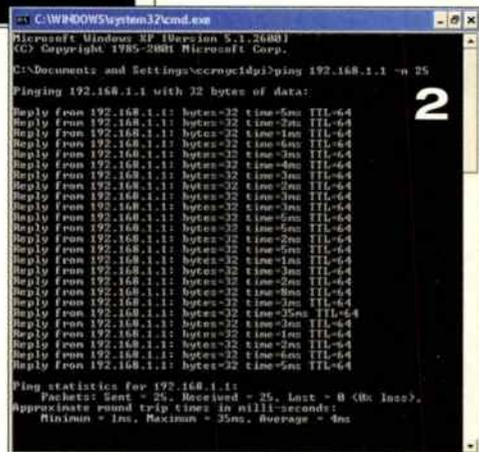
Making use of a LAN bridge of some sort (for example, a Harris/Intrplex DS-64NC) is going to slow your system down somewhat because the bridge takes a little time to decide whether or not to pass frames that your local host is generating on the transmitter site LAN over the connection to the LAN on the opposite side. This is the most likely place to have a bottleneck in terms of network's speed inbound and outbound.
