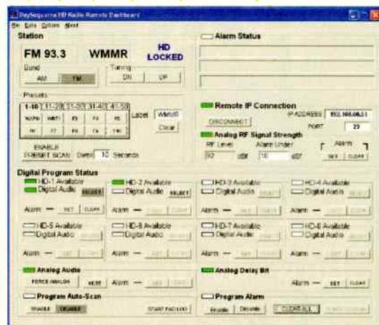
**Figure 7. The remote dashboard of the M2.2R**
