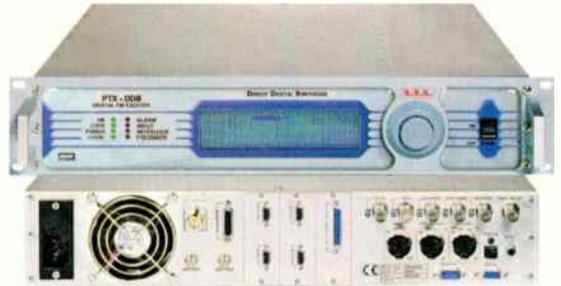
**PTX100-DDS:** PTX100-DDS uses DSP technology complying with all EC, FCC and CCIR standards. It features a built-in digital stereo coder, ITU professional limiter and on-board RDS, and AES/EBU, L/R, mono and MPX inputs, auxiliary inputs for SCA/RDS signals. It is completely microprocessor controlled, easy to program via menu or RS-232, and all main parameters are displayed on the LCD screen. It interfaces with all RVR telemetry systems to guarantee simple remote control of operating parameters.
