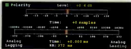
**Figure 1. Time and level alignment screen on the Belar FMHD-1**
