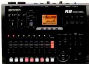
**Zoom R8:** In addition to eight-track playback and two-track simultaneous recording using SD memory cards, the R8 is a digital multi-track recorder, an audio interface, a control surface and pad sampler. The built-in drum sounds can be triggered using eight pads and three bank keys
