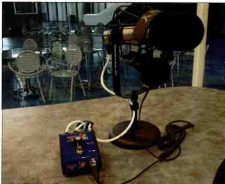
**The modified cough box and mic setup features adjustable volume and custom labeling.**
