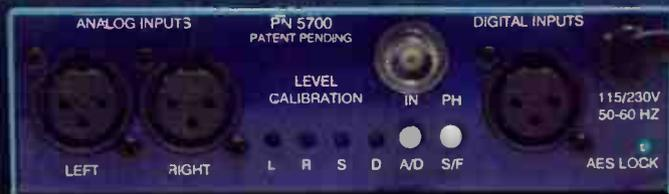
The **Stereo Audio Monitor (SAM)** is a stereo level and phase meter that incorporates Single Stereo Display\* technology. SAM provides a visual indication of the levels and phase relationships of a stereo audio signal. The unit indicates the usual Left and Right channel levels, and also displays the Sum and Difference components of the stereo signal.
