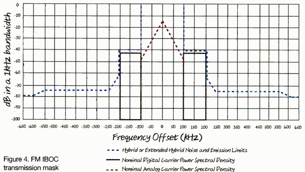
Figure 4. FM IBOC transmission mask
