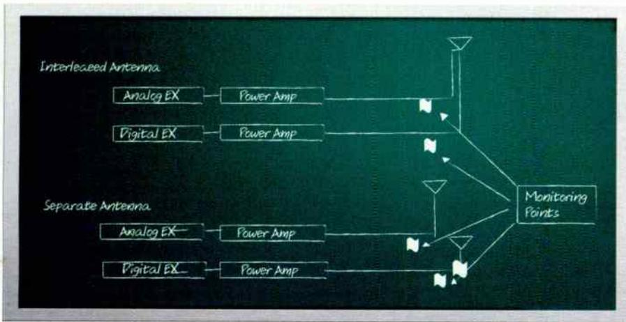
Figure 3. Separate transmitter configurations
