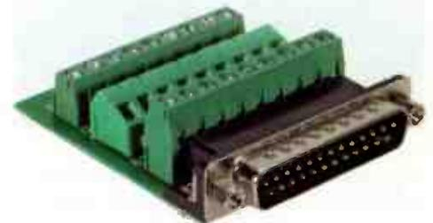
termination connectors. One notable difference between the new male connectors and existing female connectors is that L-com has rotated the male connectors' terminal blocks 90 degrees, simplifying termination because the wires will not have to be routed so many different distances. The new male connectors also have two holes at the back of the PCB to allow for a tie-wrap to lock down wire or cable.
