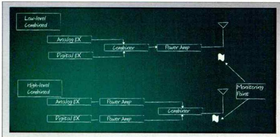
Figure 2. Combined transmitter configurations
