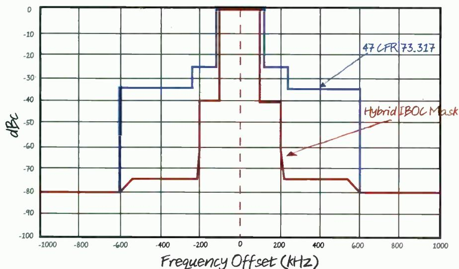
Figure 5. Comparison of FM hybrid mask and FCC mask
