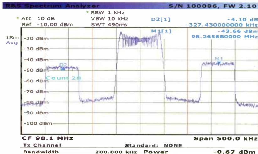
Figure 9. Asymmetric FM hybrid spectrum
