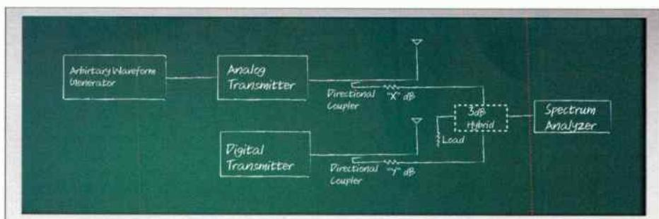
Figure 7. Measurement setup for separate transmitter configuration
