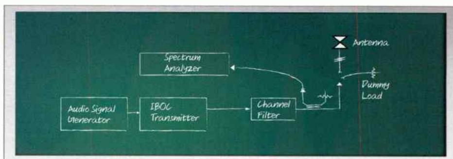
Figure 6. Measurement setup for combined transmitter operation
