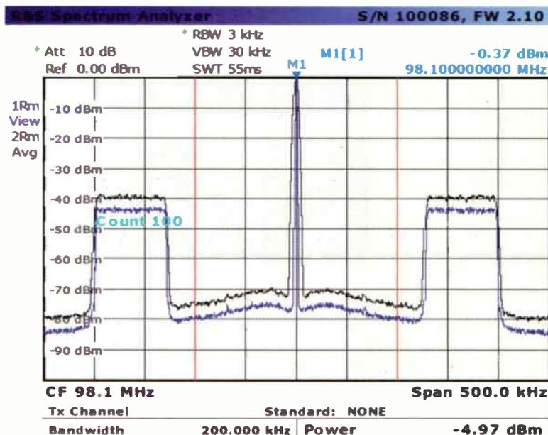
Figure 1. FM hybrid IBOC signal without modulation
