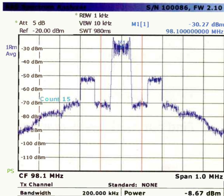
Figure 8. Combined IBOC and modulated analog signal with undesired energy.
