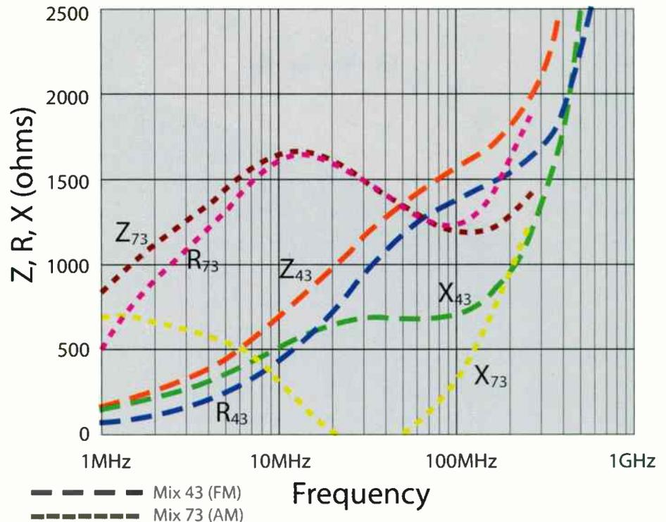
Impedance, resistance and reactance comparison for mix 73 vs. mix 43 materials.
