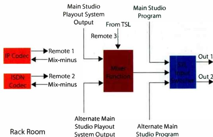
specified dayparts of automation plus satellite audio to feed the STL switch.
