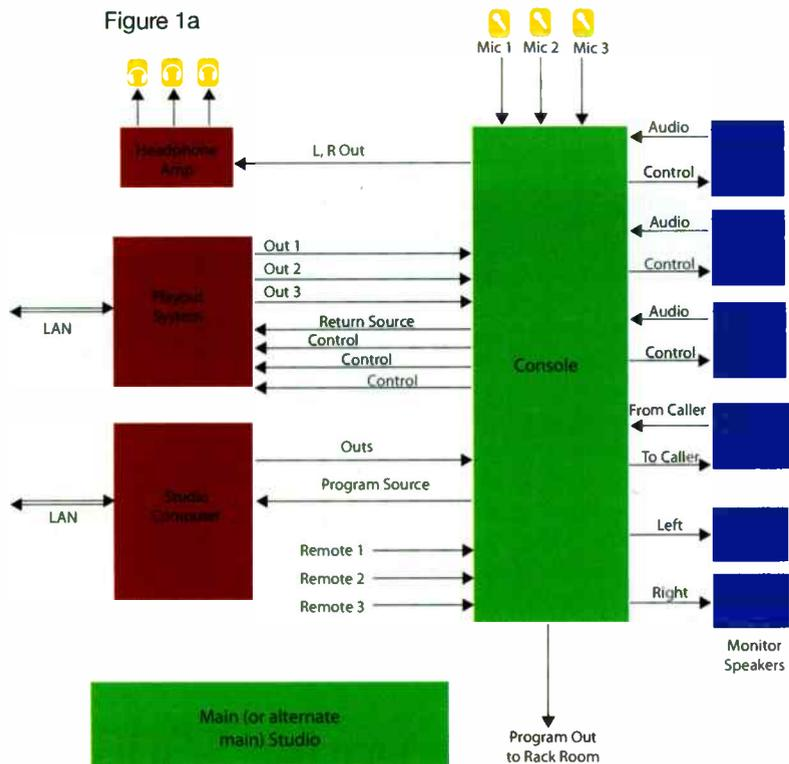
Figure 1a shows the proposed architecture. They are identical with respect to recording and playback, and the automation system is dedicated to its studio. A studio computer records and edits audio, and retrieves audio via the Internet.
